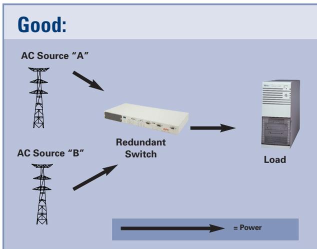
In this application, the Redundant Switch is connected to two separate AC sources. Loads with single or multiple power cords can now have N+1 power paths, to deal with a single AC source failure. The AC sources can originate from a centralized UPS, a generator set, or even separate utilities. *Protection:* This application protects against failure of one of the two AC sources. These problems can range from a tripped circuit breaker, to a utility blackout, to a centralized UPS failure.
